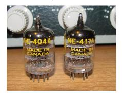
happening was that the different types of tubes were manufacture by Western Electric in the US and shipped to Canada for final assembly. This was probably done so a Made in Canada label could be placed on the tube. The labeling was done in yellow the same colour used by Western Electric. If the above is correct the Northern Electric tubes were pretty much manufactured by Western Electric in the US.
