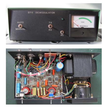
The transformer is large because it was also used for the machine's loop supply. The missing fuse was in the machine's loop circuitry. The relay is missing because later the auto start was no longer required. A computer was used in place of the machine. I think the vertical mounted perf board on the back was a serial interface for the computer. I can't quite remember.
