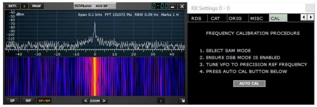
The frequency resolution is also amazing with down to **1 HZ** marks on the auxiliary spectrum display. The screen capture on the above left shows a total span width of 100 Hz with marks every Hz. The above right shows the calibration window.
