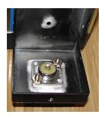
I checked the VSWR on 2 meters using a Bird 43 Wattmeter and after doing the conversion calculation it indicated about 1.5 to 1. Although the dummy load was not rated higher than 160 MHz, I checked it at 440 MHz. It was un-usable at this frequency.
