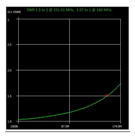
The red marker at the 1.5 to 1 SWR line is at 151.51 MHz.
