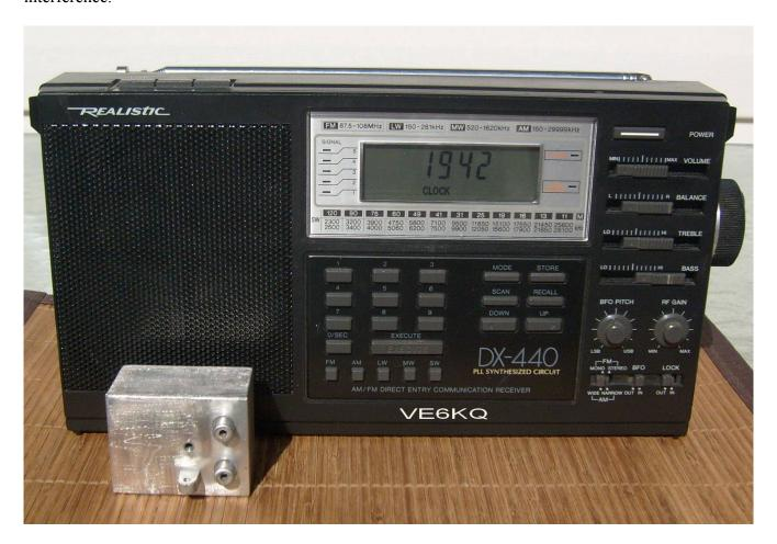
I now use it almost exclusively to monitor the 20 meter AM frequency, 14.286 MHz. There was a problem here also. When connected to a decent outside antenna it pretty much died due to front end overload from other signals. The receiver doesn't appear to have any front end selectivity. Turning down the the RF gain helped a little but not much.
