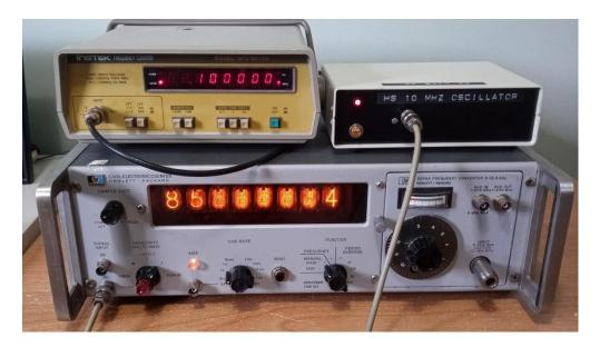
Shown is a 10 MHz signal divided down to 100 KHz. The instrument is flexible enough to allow this signal to be divided down to below 1 Hz. This feature might be useful if you had for example a GPSDO with an output of 10 MHz and you wanted a lower frequency output. The scaler seems to be independent of the instrument's time base oscillator or I don't know why this feature would have to rely on the internal time base.
