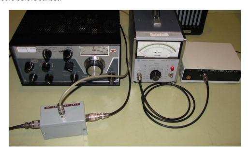
So far the stability of the oscillator seems pretty good. I calibrated it after a 2 day warm up and again about 10 days later. From what I can tell it moved a little but not very much, only a fraction of a Hertz at 10 MHz. I plan on doing long term stability tests on the oscillator.
